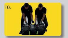
10. Fold over the packaging tarpaulin. Now use the straps to lash the safety cushion. **Do NOT knot the side tie fastening!** Tighten the straps at the corresponding strap tensioners as required.
