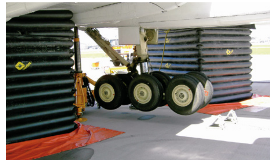
Aircraft Lifting Bags – quick and secure recovery
